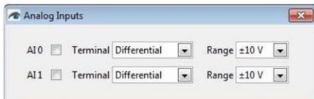
Adds analog inputs to the tester. For each channel the ground reference setting can be set to “Differential” or “Single-Ended” and the voltage range set to  $\pm 10V$ ,  $\pm 5V$ ,  $\pm 1V$  or  $\pm 0.2V$ . Signals shall be connected to the dedicated SCC-68 box that is provided to users with this software add-on. See the SCC-68 reference label inside the box and/or the SCC-68 user guide for the proper location of the inputs terminals.
