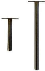
Sample Holder, T-shaped Tensile
