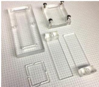
Lap Shear Test Fixtures
