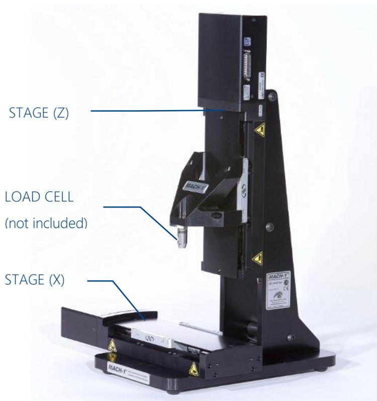
One vertical stage and one horizontal stages for compression, tension and shear testing
