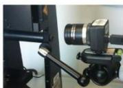
A Camera Feed can be added to the Mach-1 mechanical Tester. The live video streaming facilitates the setup of test sequences, particularly for small samples. This feature allows the capture of series of high definition images of the sample during mechanical testing. Image capture is synchronized with the raw data of the mechanical test. These images can be easily exported to third-party software for image processing. For example, they can be exported to Matlab® for deformation field analysis.
