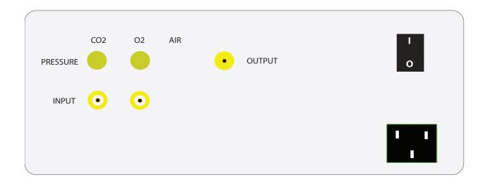
Turn the controller ON. The controller will self-calibrate itself for 5min. After 5min, the display will show concentrations of CO2 and O2 in the output mixture and start making the mixture according to factory settings of 5% CO2 and 20% O2.
